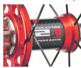
When you push on the pedals, the rotational force on the sprocket induces a slackening of the freewheel spokes with a consequent loss of rim tension. This results in undesirable flex of the whole wheel and an unavoidable loss of energy. Fulcrum® has solved this classic cycling problem with its 2:1 Two-to-One™ Spoke Ratio patent, by doubling the spokes in the critical zones.
